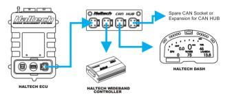
B. Haltech CAN Devices and Expansion to Second CAN Hub
